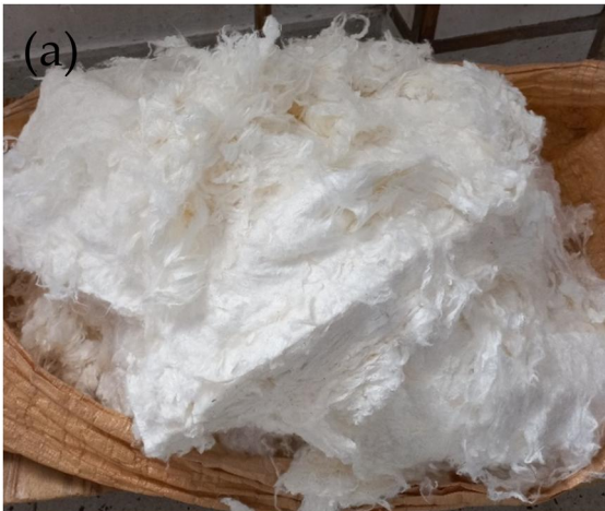
Figure 1. (a) Viscose rayon as a host fiber and (b) polyester as a neppy fiber.
