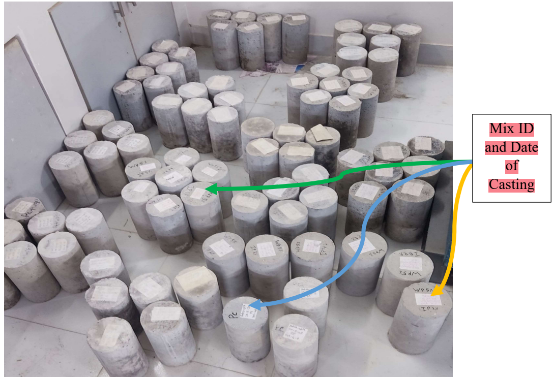
Fig. : Demolded Concrete Specimens with Identification Mix ID and Date of Casting.
