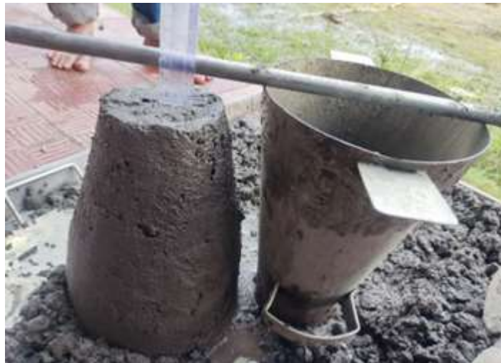
Fig.: Workability Test (Slump Test)
