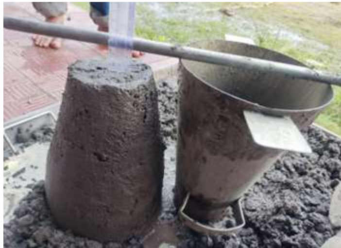
Fig. : Workability Test (Slump Test).
