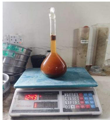
Fig. : Specific gravity test of Wood dust (WD)
