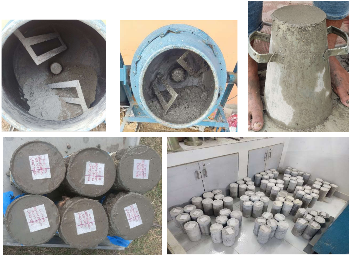
Fig , : Concrete Casting Step by Step following ASTM C192/C192M-19 (ASTM, 2022)
