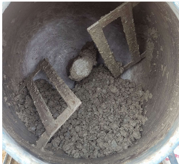
Fig. : In dry mix after adding water in concrete.
