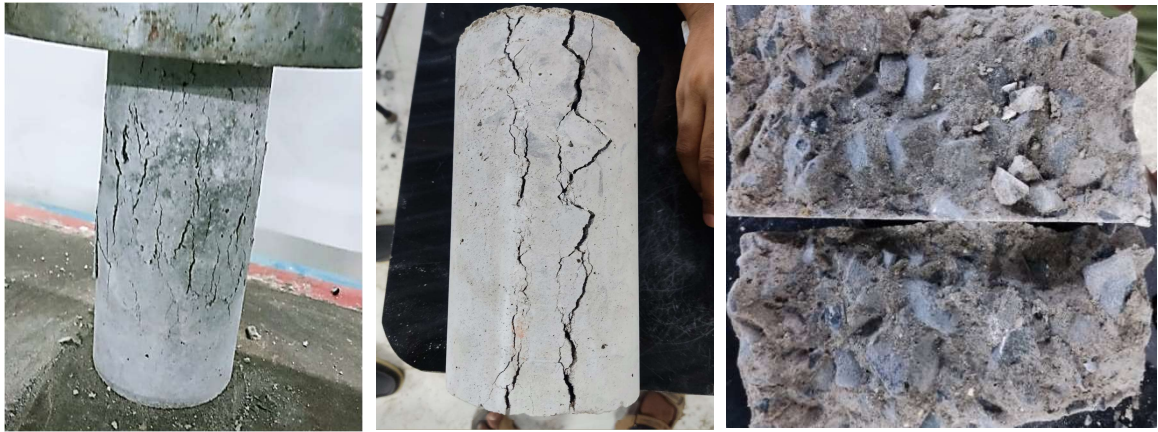
Fig. : M4 specimen under compressive & splitting tensile strength test failure
