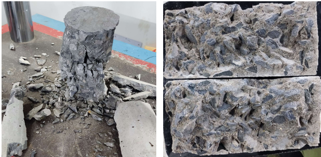
Fig. :Control specimens compressive & splitting tensile strength test (brittle) failure.
