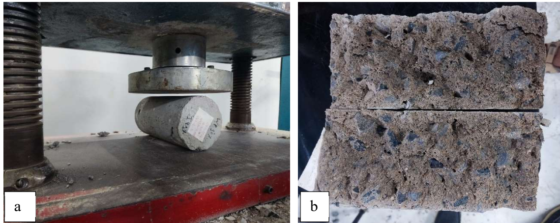
Fig. : Splitting Tensile Strength Test Performed by (Universal Testing meshing , UTM) (ASTM C496) a)Before applying load ,b)After applying load.
