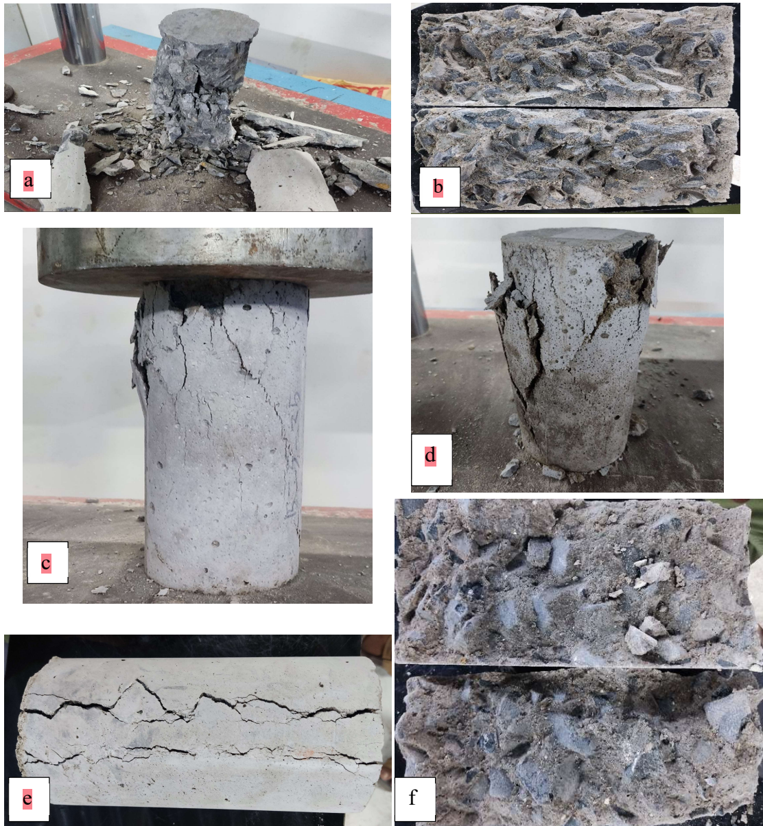
Fig. : Different Failure / Crack Pattern . a) M1 at Compressive strength tests, b)M1 at Splitting Tensile Strength test ,c)M11 at Compressive strength tests, d)M14 at Compressive strength tests, e)M4 at Splitting Tensile Strength test, f) M13 at Splitting Tensile Strength test.
