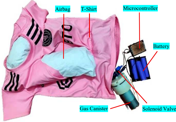
Fig 4. The smart wearable prototype with an integrated airbag safety system.
