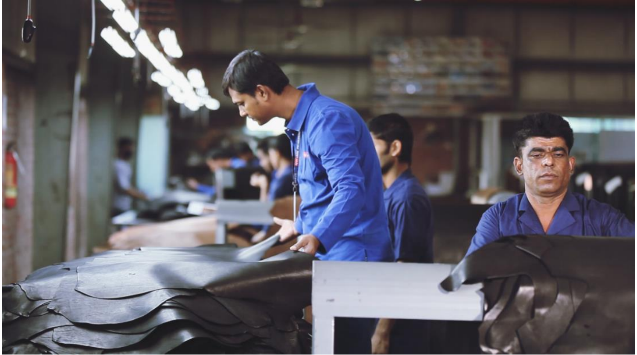
Pic: Inspection of qualityful leather before cutting
