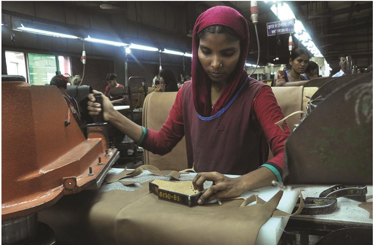
Pic: Inspection of qualityful leather before cutting
