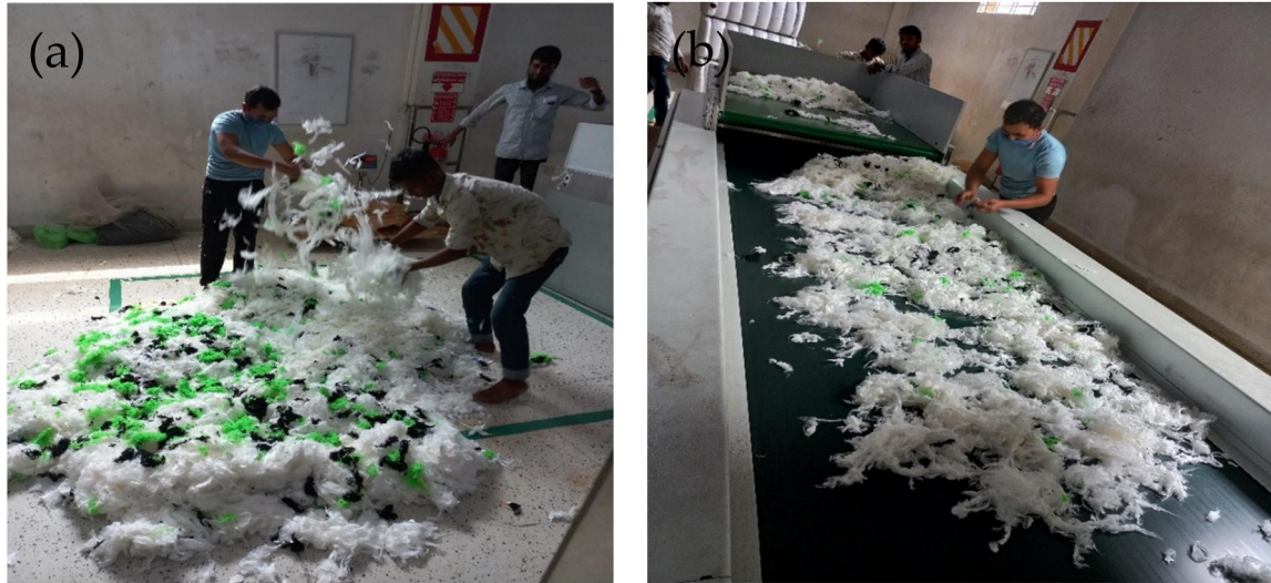
Figure 2. Processes for blending neppy fiber with host viscose rayon fiber: (a) hand mixing and (b) manual bale opener.
