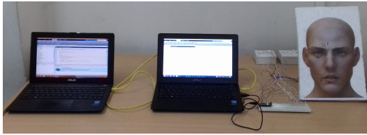
Fig. 4: Overall setup (from left to right: sender PC, physical link, receiver PC, Arduino, Robotic face).
