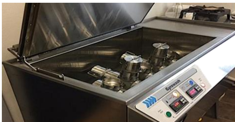
Figure 1. Apparatus for fabric wash fastness test
