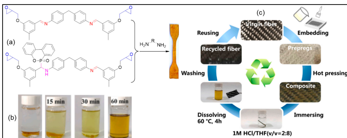
Figure 19. (a) Preparation of biobased imine bond-containing ER; (b) graphical presentation of degraded ER in acidic solution over time and (c) closed-loop recycling of carbon fibre composite [Reproduced with permission from Yang et al.; published by Elsevier, 2022] [102].
