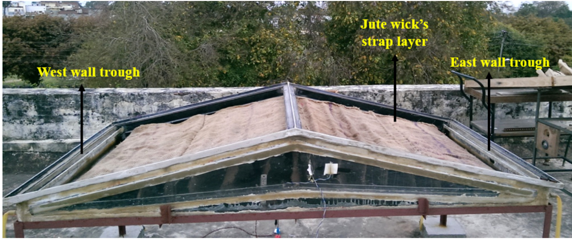
Fig. 2. Photograph of the solar still showing south wall's trough and pattern of hanging wicks.
