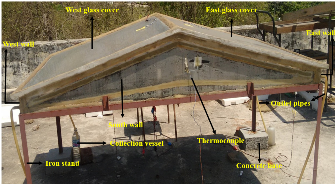
Fig. 3. Photograph of the solar still.
