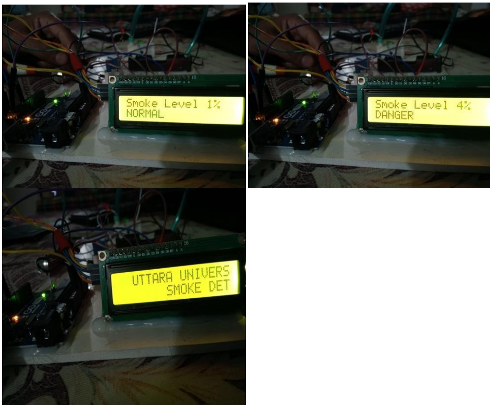
Figure: SMOKE, GAS & SMELL DETECTOR PROJECT
