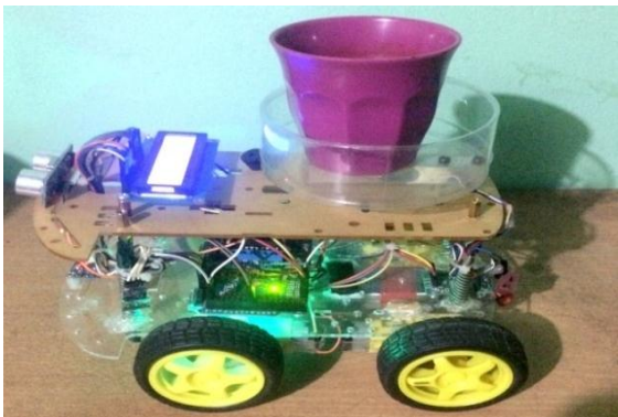
Figure 7. Complete setup of a robot waiter with a cup of drink
