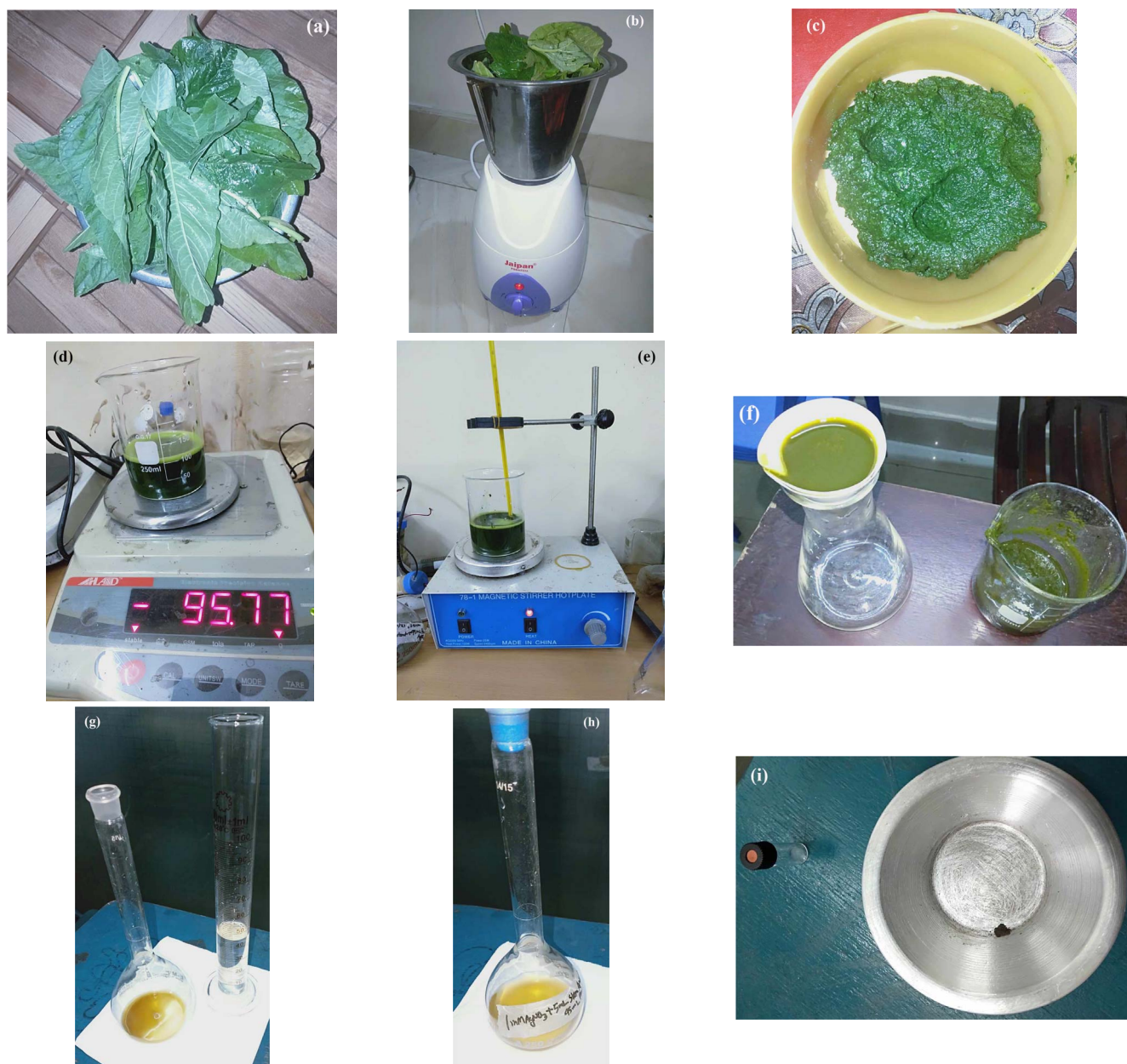
Figure 1. Steps: (a) Fresh red amaranth, (b) Mixing red amaranth in a blender, (c) Mashed red amaranth, (d) Mashed red amaranth with de-ionised water, (e) Heating at 62 °C for 60 min with a magnetic stirrer with a hot plate, (f) Filtrating red amaranth extract with Whatman paper, (g) \text{AgNO}_3 and filtered red amaranth extract, (h) Ag NPs are synthesised using red amaranth extract, and (i) The powder form of Ag NPs), as shown in the diagram.
