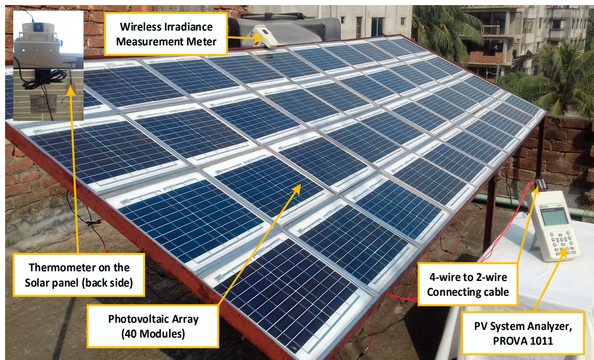
Figure 12. Experimental setup of 400 W array for comparing maximum array output power using different methods of modules arrangement.
