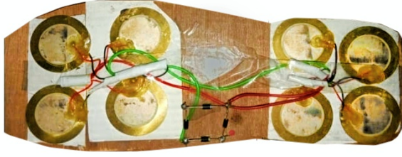
Fig. 5. Experimental Setup of eight unit piezo sensors connected in parallel configurations
