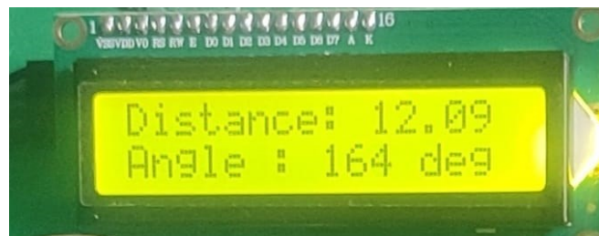
Figure 17: The result of system is represented by LCD Display, short distance, angle view
