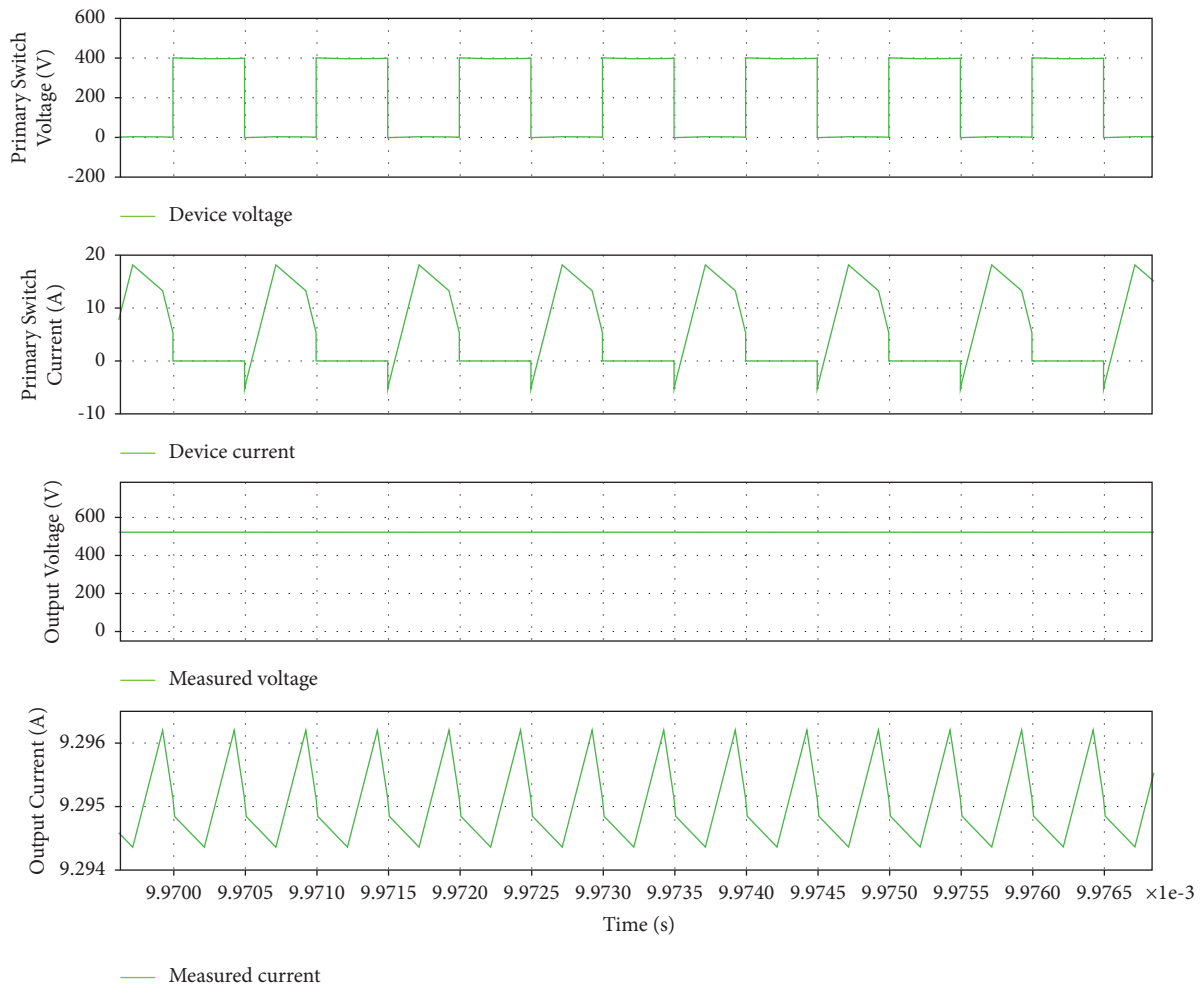
FIGURE 15: Simulated waveforms for the Si power transistor-based converter.
