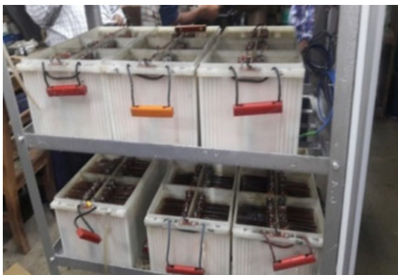
Fig. 5 An experimental setup of a 1-KW PKL power production from the PKL extract
