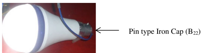
Fig. 4 LED bulb lights with self-short-circuit condition
